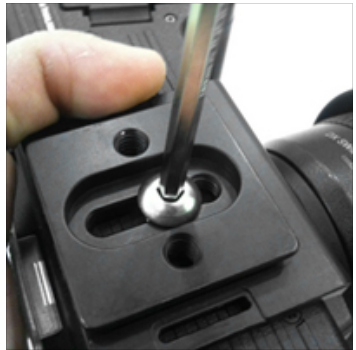
6. Slide the plate so that the flange is flush against the body. Tighten the bolt.
