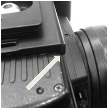
5. Slide the plate that there is no gap between the flange and the camera body.
