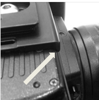
7. Make sure that there is no gap between the flange and the camera body.
