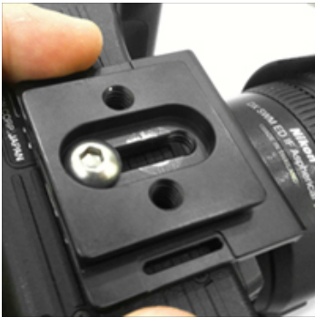
4. Screw in but not tighten the bolt to the body while leaving one or two turns.
